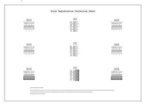
**6** Find the location on each chart where 2 lines most closely overlap each other. If this is the 0 position, registration for that color is not required. For the illustration, B is the appropriate value.
